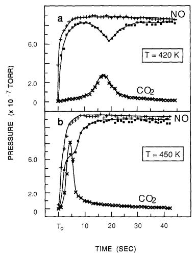
Fig. 2. The NO (+ and  $\blacksquare$ ) and CO<sub>2</sub> (×) signals monitored during the titration of preadsorbed CO by NO at (a) 420 K and (b) 450 K.
