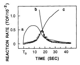
FIG. 6. Models for the CO<sub>2</sub> production rate for the titration of preadsorbed CO by NO at 420 K. Shown are the experimental data points ( $\square$ ), the bimolecular rate law,  $R_{\text{CO}_2} = k\theta_{\text{NO}}\theta_{\text{CO}}$  (curve a), the ( $\theta_{\text{CO}}$ )<sup>2</sup> expression (curve b), and the dissociative rate law,  $R_{\text{CO}_2} = k'\theta_{\text{NO}} \cdot S$ , resulting from a NO dissociation rate-limiting step (curve c).
