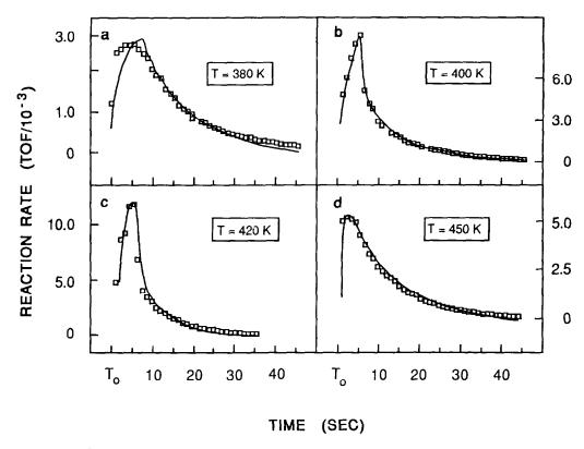
Fig. 5. Summary of the  $CO_2$  production rates ( $\square$  indicates experimental data points) modeled using the bimolecular and dissociative rate expressions for the titration of NO by CO experiments at (a) 380 K, (b) 400 K, (c) 420 K, and (d) 450 K.
