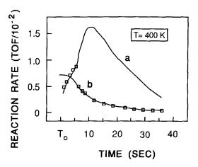
Fig. 4. Models for the CO<sub>2</sub> production rate for the titration of preadsorbed NO by CO experiments at 400 K. Shown are the experimental data points ( $\square$ ), the bimolecular rate law,  $R_{\text{CO}_2} = k\theta_{\text{NO}}\theta_{\text{CO}}$  (curve a), and the dissociative rate law,  $R_{\text{CO}_2} = k'\theta_{\text{NO}} \cdot S$ , resulting from NO dissociation as the rate-limiting step (curve b).
