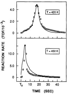
Fig. 7. Summary of the modeling of the CO<sub>2</sub> production rate for the titration of CO by NO at (a) 420 K and (b) 450 K using the dissociative ( $R_{\rm CO_2} = k'\theta_{\rm NO} \cdot S$ ) and ( $\theta_{\rm CO}$ )<sup>2</sup> expressions ( $\square$  denotes experimental data points).
