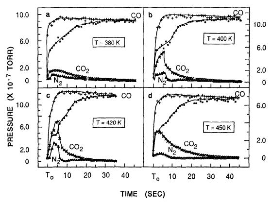
Fig. 1. The CO (+ and  $\blacksquare$ ), CO<sub>2</sub> (×), and N<sub>2</sub> ( $\triangle$ ) signals monitored in the transient experiment where preadsorbed NO was titrated by CO at (a) 380 K, (b) 400 K, (c) 420 K, and (d) 450 K.
